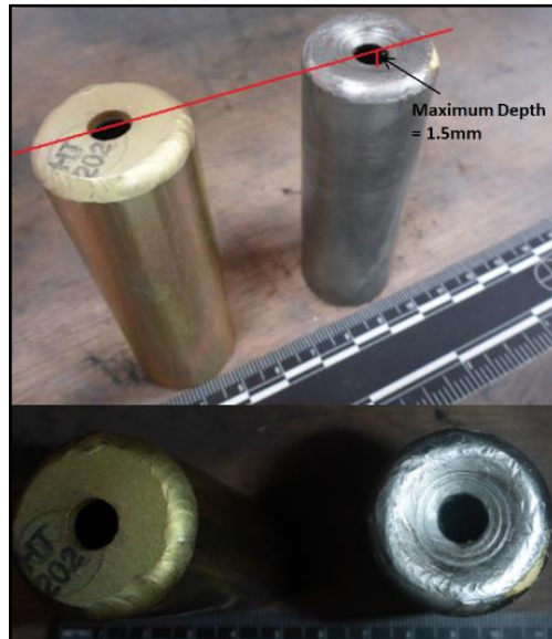
Photo No. 9: New retainer tube (gold-coloured) and old retainer tube
