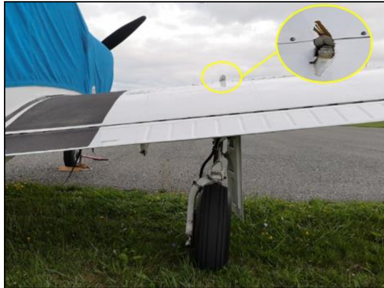
Photo No. 2: Top of undercarriage strut protruding through the wing surface
